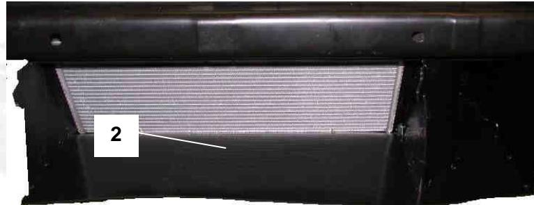
Connect the right bulkhead (ref. 3) to the lower bulkhead (ref. 2) using rilsans. Some adjustments may be necessary.
