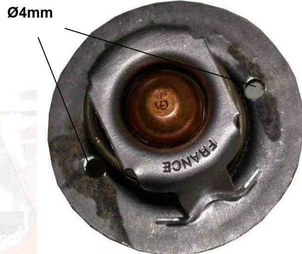
Put the new seal on the thermostat ([ref. 6](#)), and put the thermostat back on the water pipe.
