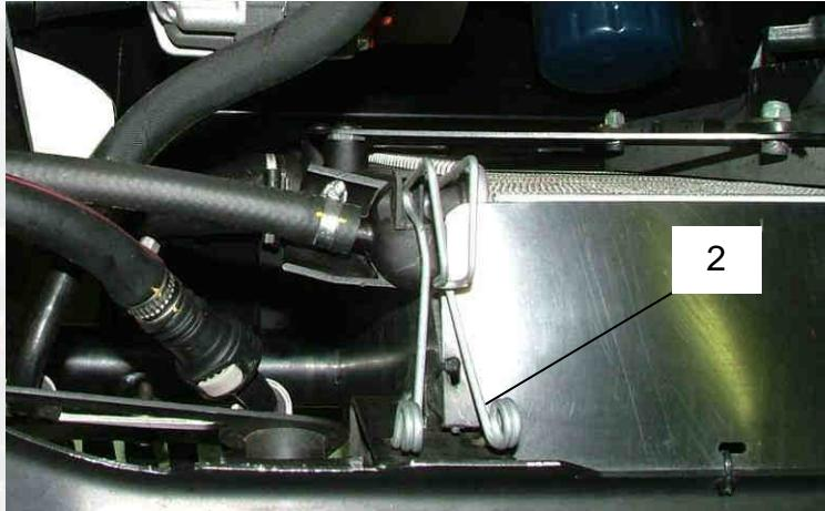
Clip the radiator using two pins, in the housings provided for this purpose (see photo below):
