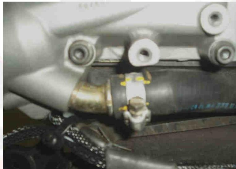
Connect the two heater hoses to the bulkhead grommet.
